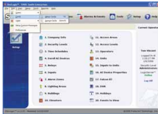
Figure 10-1 Setup Screen - From the Menu Bar, select Edit. From the drop down menu, select Cards and then Setup Cards.
