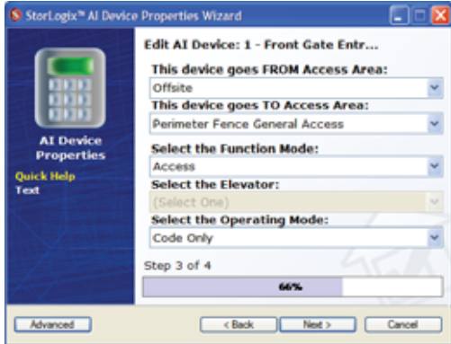
Figure 8-4 Setup AI Device Properties Wizard Step 3 of 4 - Select the From and To Access Areas, Function Mode, Elevator if applicable, and the Operating Mode. Click Next to continue.
