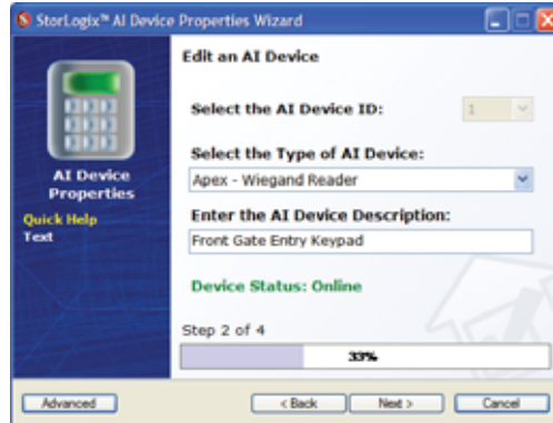
Figure 8-3 Setup AI Device Properties Wizard Step 2 of 4 - Select the type of AI Device and then enter a description for the device. Be descriptive to help with event location in the future. Click Next to continue.
