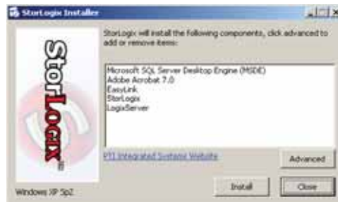
Figure 2-2: StorLogix Installer Components Screen. Components shown will be installed. To change this list or to add other components, click on the Advanced button.
