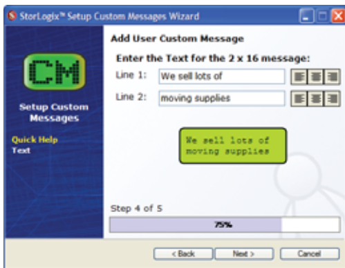
Figure 10-17 Setup Custom Messages Wizard Step 4 of 5 - Enter the text as the message will appear on a VP keypad. Then click Next.
