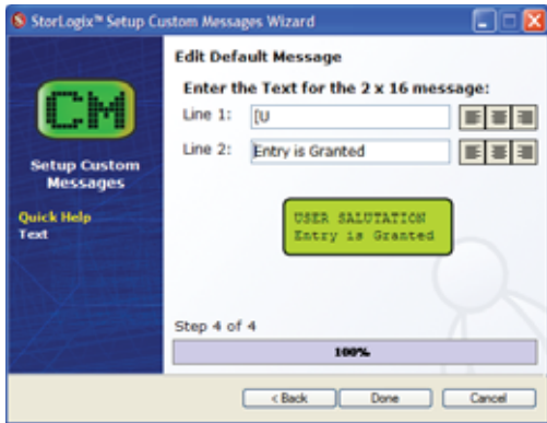
Figure 10-11 Setup Custom Messages Wizard Step 4 of 4 - Enter the text as the message will appear on an VP keypad. Then click Done.
