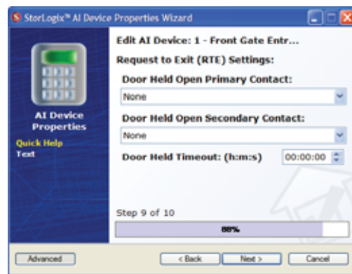
Figure 8-11 Setup AI Device Properties Wizard Advanced Step 9 of 10 - Select the Request to Exit Door settings. Click Next.
