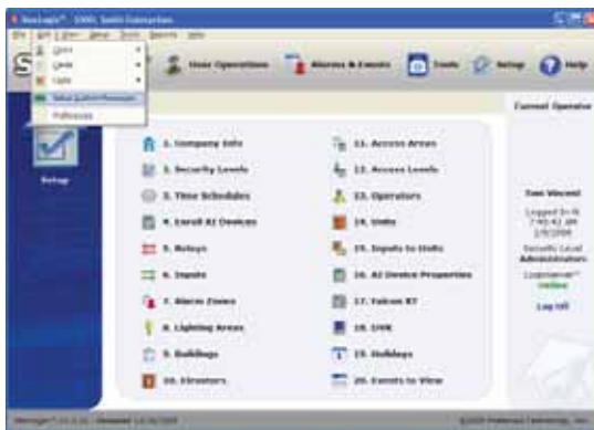
Figure 10-7 Setup Screen - From the Menu Bar, select Edit. From the drop down menu, select Custom Messages.
