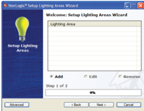
Figure 5-9 Setup Lighting Areas Wizard Step 1 of 2 - select Add to add a new lighting area or select a lighting area from the existing list and click on edit to edit the Lighting Area and Remove to remove it. Click Next to continue.
