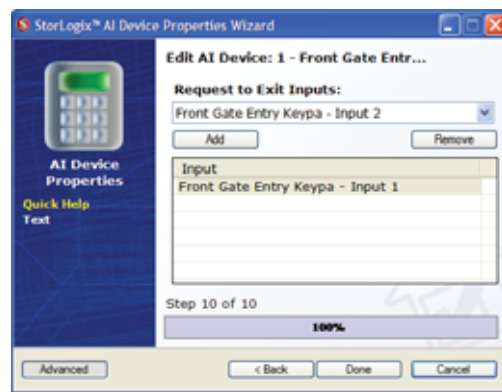
Figure 8-12 Setup AI Device Properties Wizard Advanced Step 10 of 10 - Select the Request to Exit Door Inputs. Then click Done.
