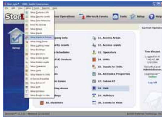
Figure 10-35 StorLogix Main Screen - Select Setup on the Menu Bar and then Setup Inputs to Relays from the drop down menu.
