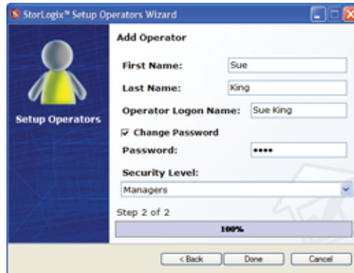
Figure 6-17 Setup Operators Wizard Step 2 of 2 - Enter the operator information and click Done.
