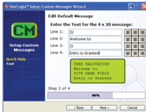
Figure 10-10 Setup Custom Messages Wizard Step 3 of 4 - Enter the text as the message will appear on an Apex keypad. Then click Next.
