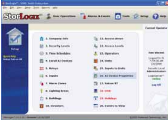
Figure 10-22 StorLogix Setup Screen - Select 16. AI Device Properties to set a custom message for a keypad.
