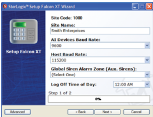
Figure 8-14 Setup Falcon XT Wizard Step 1 of 2 - Change the Site Name and Baud Rates if needed. Set the Global Siren Alarm Zone and Log Off Time of Day as necessary.
