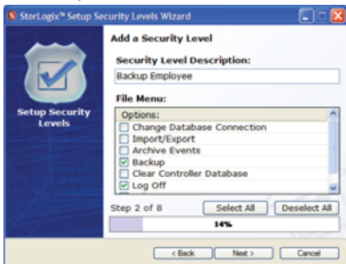
Figure 3-28: Setup Security Levels Wizard Step 2 of 8 - Review the File Menu options to check any that operators in this security level should have access to or uncheck any that they should not have access to.
