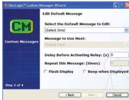
Figure 10-9 Setup Custom Messages Wizard Step 2 of 4 - Select the message to edit, set the delay, repeat, flash, and beep functions. Then click Next.
